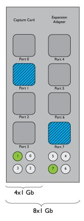
**Note:** The 2 x 10 Gb adapter assigns the numbers 0 and 1 to the ports, in order from top to bottom.
