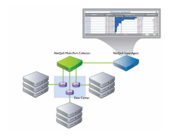
Depending on the type of configuration you purchased, a single Multi-Port Collector network interface card can be connected to SPAN ports on as many as eight separate switches. During NetQoS SuperAgent configuration, you add the Multi-Port Collector as a collection device. Data from the monitored switches is sent to the SuperAgent Management Console within a few minutes, where it is included in all SuperAgent reports.
