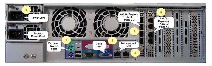
The image shows the back of the Multi-Port Collector appliance in the **8 x 1 Gb** configuration (which has two 4-port adapters). The basic cabling steps are the same for the other two types of Collector configuration. The numbered labels show where you must plug in the following components:
