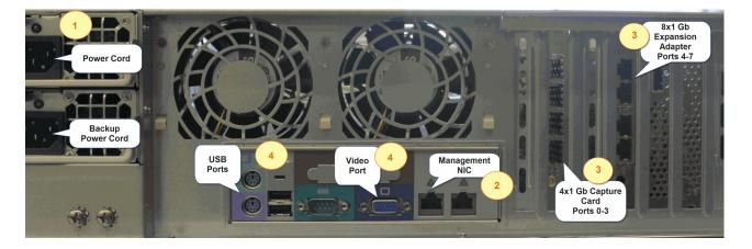
The image above shows the back of the Multi-Port Collector appliance in the  $8 \times 1 \text{ Gb}$  configuration (which has two 4-port adapters). The basic cabling steps are the same for the other two types of Collector configuration. The numbered labels show where you must plug in the following components:
