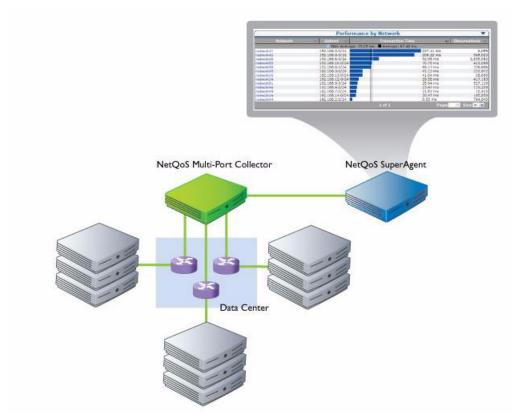
Depending on the type of configuration you purchased, a single Multi-Port Collector network interface card can be connected to SPAN ports on as many as eight separate switches. During NetQoS SuperAgent configuration, you add the Multi-Port Collector as a collection device. Data from the monitored switches is sent to the SuperAgent Management Console within a few minutes, where it is included in all SuperAgent reports.
