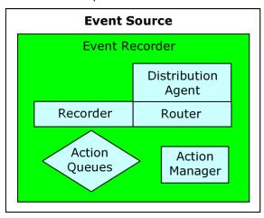
The eTrust Audit client is installed on an event source (in green) and contains routing and filtering components (shown in blue).
