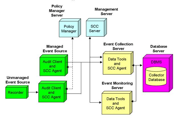
Typically there are many different event sources, both managed and unmanaged. A managed event source has client components installed and processes events using policies from the Policy Manager. If you are using eTrust Security Command Center, you can also install an SCC Agent on the managed event source to gather operational status information.
