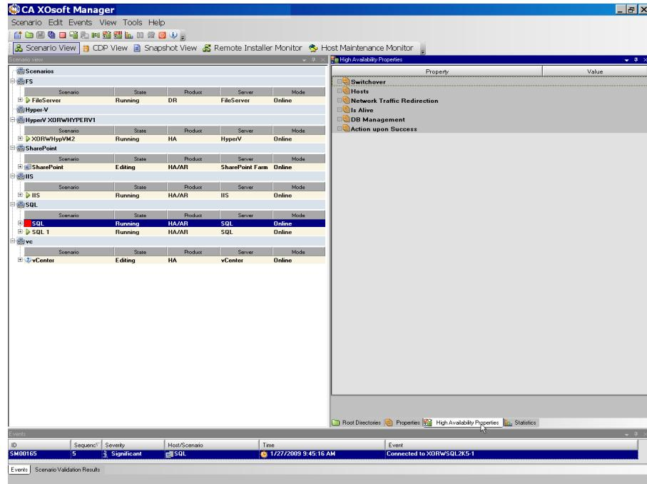
2. Expand Hosts. Verify that the Master Full Qualified Name is the correct DNS name for the SQL Server to which the BES servers connect.
