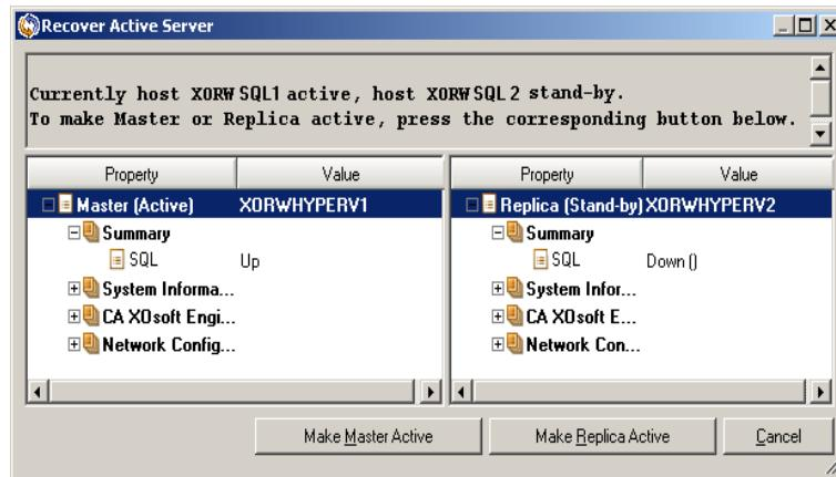
**Important!** If a legitimate switchover in a disaster situation occurs and users are redirected to the Replica server for any period of time, it is important to replicate all changes on the Replica back to the Master before making the Master server active. Using *Recover Active Server* in such a situation results in loss of data.
