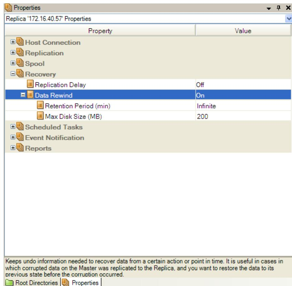
If this option is set to Off, the system will not register data rewind points. For more information about Data Rewind parameters (Retention Period, Max Disk Size), see the *CA XOsoft User Guide*.
