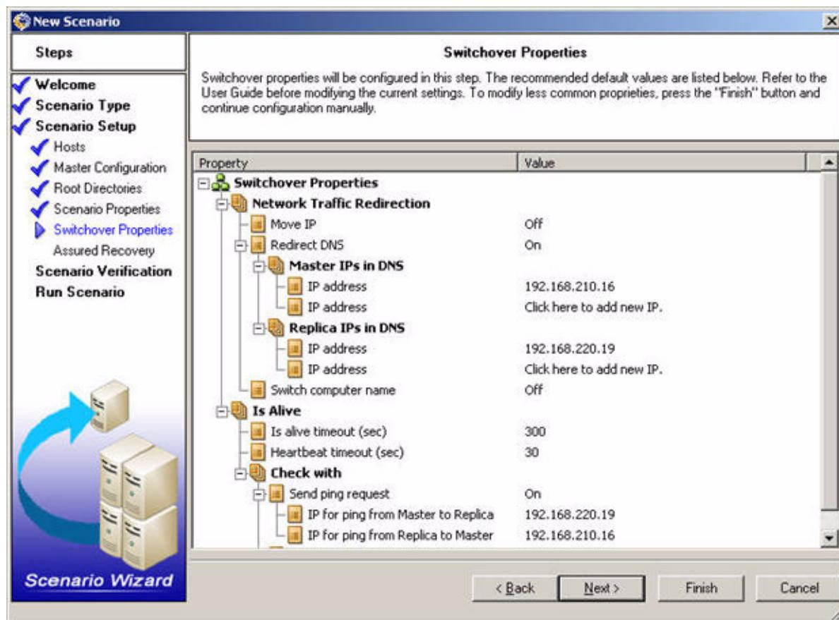
9. The last step in Switchover Properties defines which steps are triggered automatically by WANSyncHA or triggered manually by the Administrator. Select the desired setting for each option and then click the Next button.
