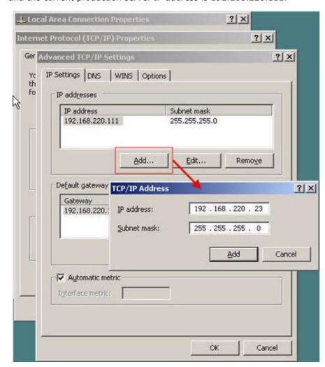
Note that in the following screen shot, the WS-IP IP address is 192.168.220.23 and the current production server IP address is 192.268.220.111.
