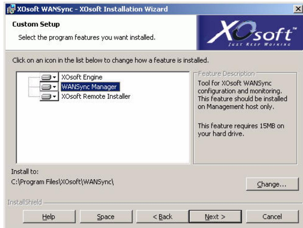
If you intend to use the XOsoft Remote Installer (recommended), the machine on which you are running the remote installer must have the .Net framework 2.0 installed. The framework is required only on the machine running the remote installer wizard (GUI); the target servers do not have this requirement.
