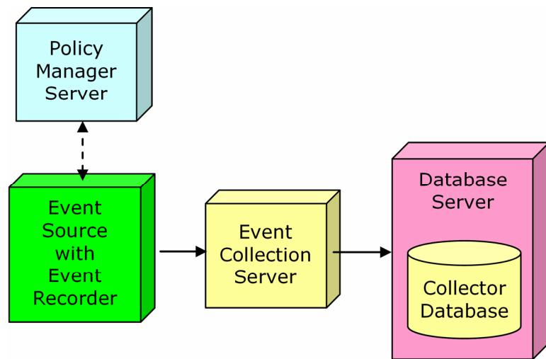
The database (DBMS) should be located on a dedicated server. The separate event collection server supports a Collector service and other data tools. Separation of these two machines provides better performance. For very large networks with high event volumes, a storage network array such as a Storage Area Network (SAN) may be a better alternative for event storage.
