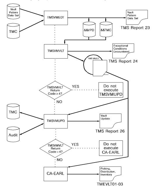
The following diagram provides an illustration of a VMS Program Execution:
