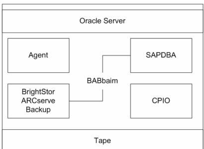
The following diagram shows how a SAP R/3 database is backed up when BrightStor ARCserve Backup is installed on a local server:
