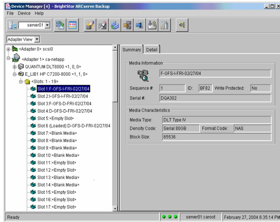
**Note:** If you want BrightStor ARCserve Backup to use tape devices attached to NAS servers, you must run `camediad_setup`, to first configure those devices with BrightStor ARCserve Backup.
