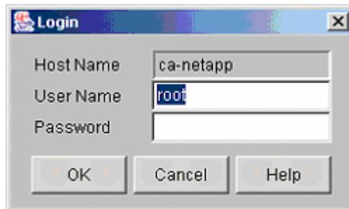
5. Enter the user name and password for the account that has access to the NAS filer and click OK. The volumes and files on the NAS filer display.
