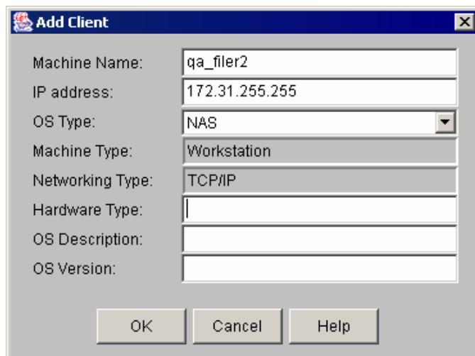
3. Add the NAS server's machine name and IP address.
