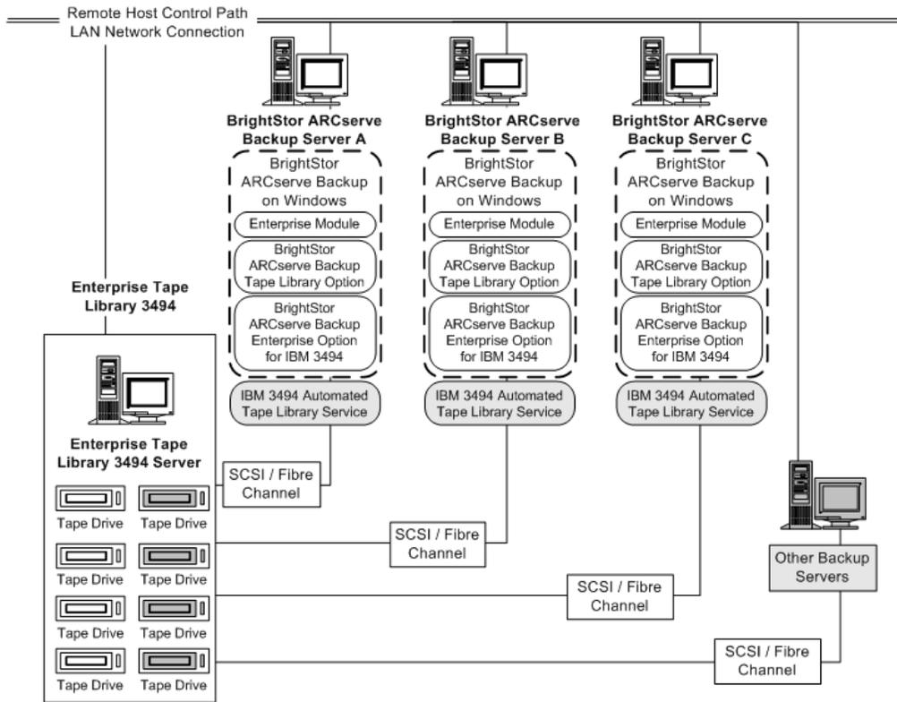
If multiple backup servers are sharing the same Enterprise Tape Library 3494, you must ensure that each tape volume is assigned to only one backup server. The tape volumes assigned to each backup server should be mutually exclusive, which means they cannot be used or accessed by other backup servers attached to the network.
