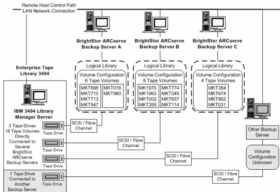
The example shows that the Enterprise Tape Library 3494 has four tape drives directly attached to several backup servers on the network. The unique tape volume assignments for each BrightStor ARCserve Backup server are:
