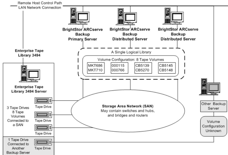
The example shows that the Enterprise Tape Library 3494 has three tape drives directly attached to a SAN. The tape volume assignments are the same for each BrightStor ARCserve Backup server in the SAN. Another backup server on the network that is not running BrightStor ARCserve Backup may have a different configuration.
