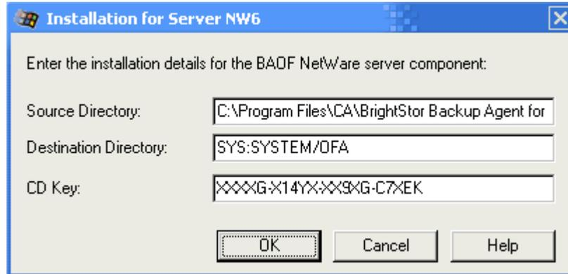
The dialog displays the source directory (the directory in which the installation files are stored) and the destination directory (the directory on the target computer in which the agent will be installed). If necessary, you can change these directory names.
