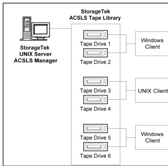
**Note:** In configurations where more than one tape drive is connected to a CA ARCserve Backup server, both tape drives must use media of the same type.
