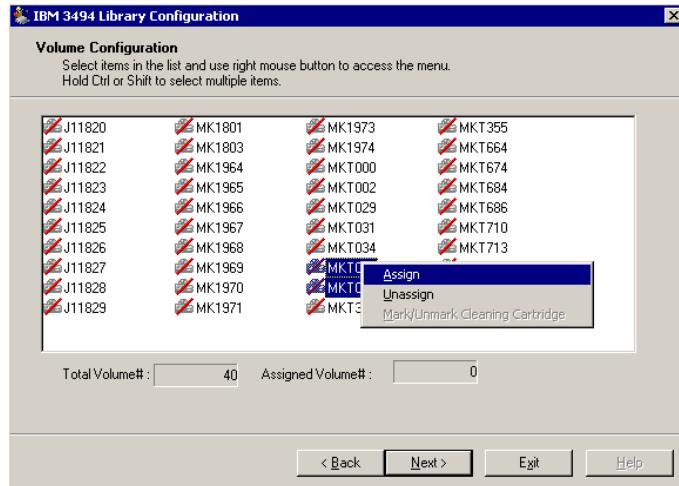
**Note:** Initially the tape volumes are not assigned to the CA ARCserve Backup server. The unassigned status is indicated by a red slash through the tape volume icon.
