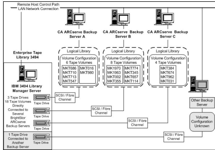
The example shows that the Enterprise Tape Library 3494 has four tape drives directly attached to several backup servers on the network. The unique tape volume assignments for each CA ARCserve Backup server are:
