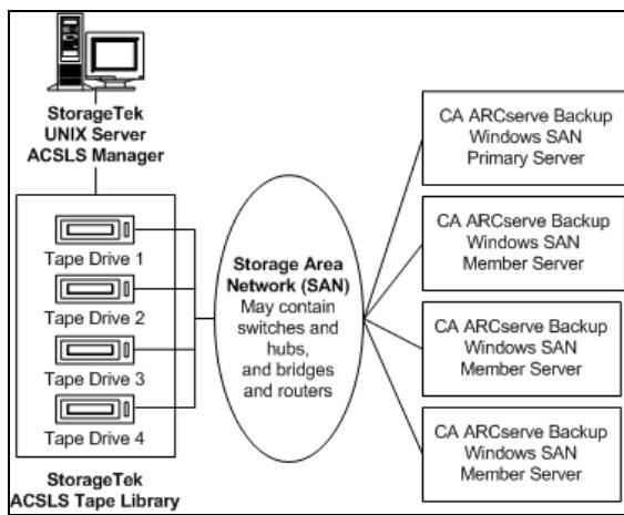
**Note:** In configurations where more than one tape drive is connected to a CA ARCserve Backup server, both tape drives must use media of the same type.
