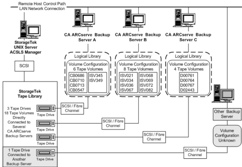
The example shows that the StorageTek ACSLS tape library has four tape drives directly attached to several backup servers on the network. The unique tape volume assignments for each CA ARCserve Backup server are:
