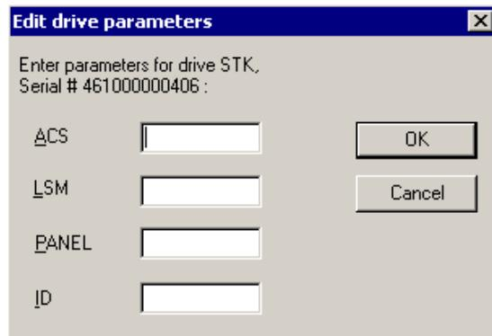
5. Enter the ACS, LSM, Panel, and ID of the tape drive in the Edit drive parameters dialog.
