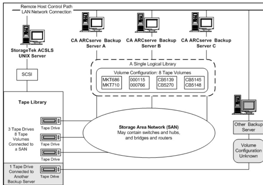
The illustration shows that the StorageTek ACSLS tape library has three tape drives directly attached to a SAN. The tape volume assignments are the same for each CA ARCserve Backup server in the SAN. Another backup server on the network that is not running CA ARCserve Backup may have a different configuration.
