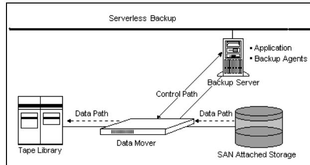
The Serverless Backup Option uses data movers to transfer data between media. This eliminates the need for moving the data to the server, and achieves the shortest data path. Data movers enhance the backup performance considerably, and yield the highest possible backup and restore speeds.
