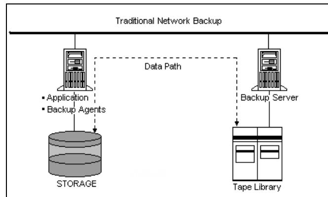
Typically, when backup operations are in progress, application processing on servers is impacted. This is one of the reasons for which system administrators prefer to perform backup operations at a time when the application load on the server is at a minimum.
