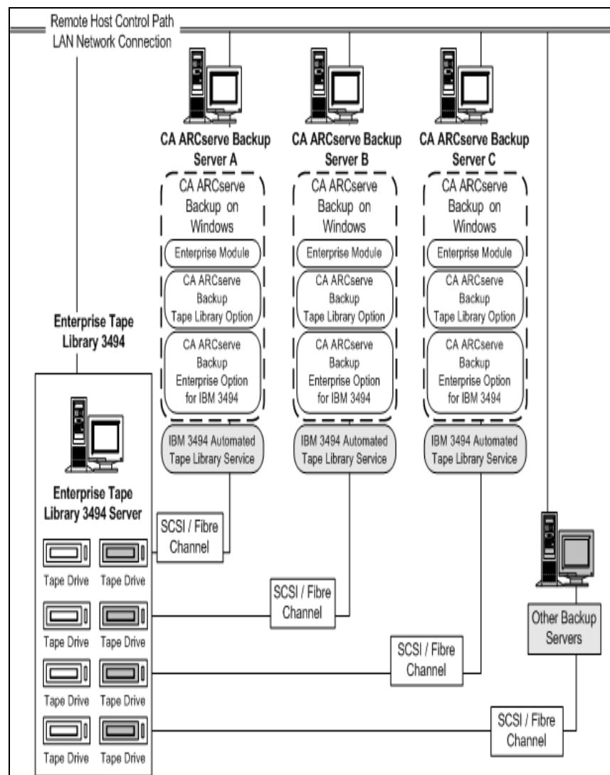
If multiple backup servers are sharing the same Enterprise Tape Library 3494, you must ensure that each tape volume is assigned to only one backup server. The tape volumes assigned to each backup server should be mutually exclusive, which means they cannot be used or accessed by other backup servers attached to the network.
