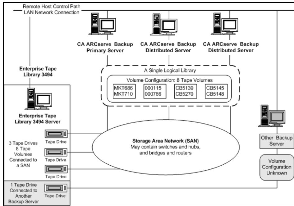
The example shows that the Enterprise Tape Library 3494 has three tape drives directly attached to a SAN. The tape volume assignments are the same for each CA ARCserve Backup server in the SAN. Another backup server on the network that is not running CA ARCserve Backup may have a different configuration.
