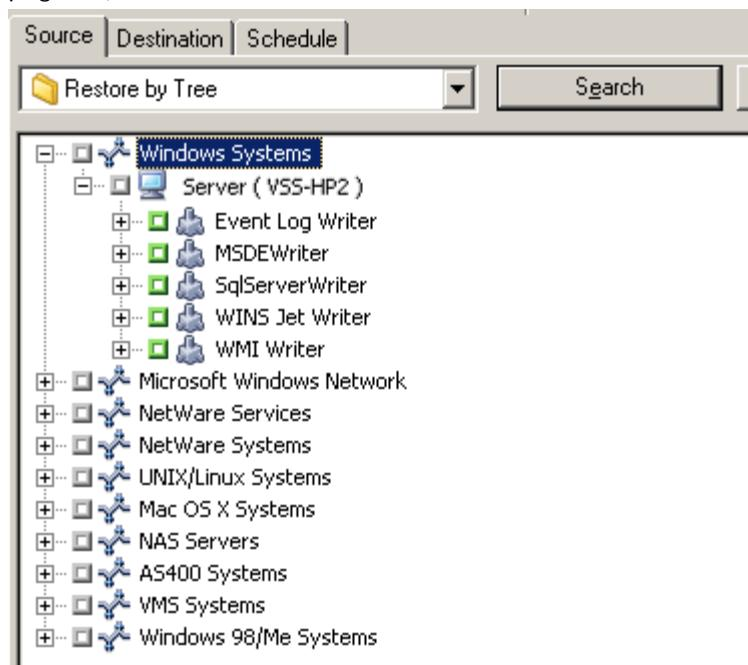
2. Click the green marker next to the name of the Writer to be restored to select it. To restore individual components, expand the Writer node and select the Components you want to restore.
