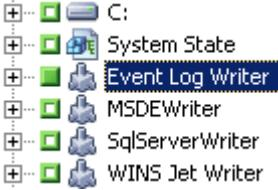
If necessary, you can expand the Writer node to view its Components. If a Writer has only one component, the marker next to its name is gray, indicating that it cannot be removed from the backup. If a Writer has multiple Components, you can, typically, choose the Components to back up. The Writer decides whether the backup of a Component is optional. Some Writers may require all Components to be backed up.
