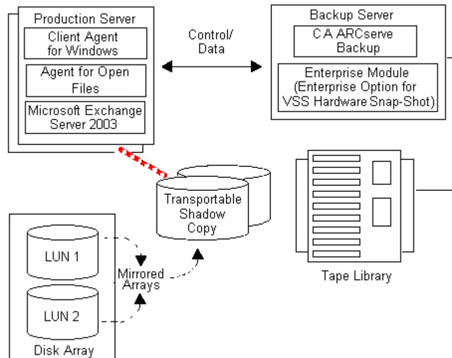
During backup operations, CA ARCserve Backup (the Requestor) contacts VSS on the production server and informs it to begin the transportable shadow copy process. VSS tells the Writer to prepare the data for the shadow copy.
