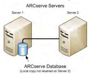
In the following diagram, multiple CA ARCserve Backup servers are sharing a centralized database. A copy of the CA ARCserve Backup database is retained on one of the servers sharing the database.
