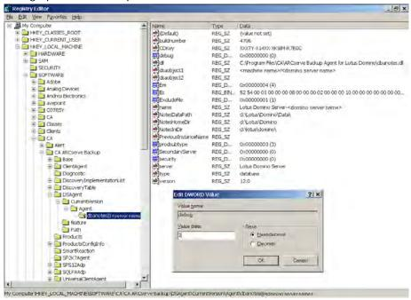
3. Set the debug parameter value to 2 to generate detailed trace files.
