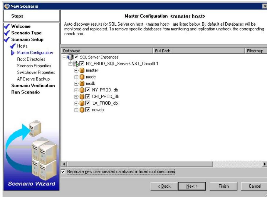
The Master Configuration screen displays all SQL Server databases for the master host, along with a check box for the "Replicate new user created databases in listed root directories" option.
