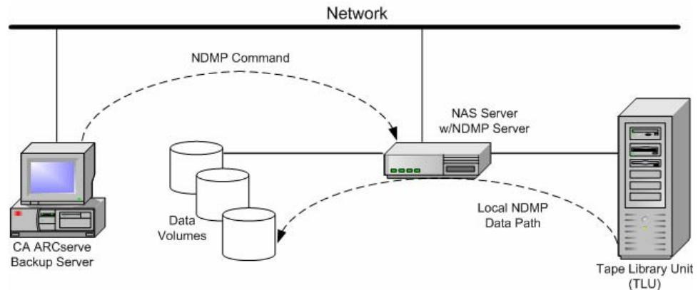
The following diagram shows an example of a three-way restore:
