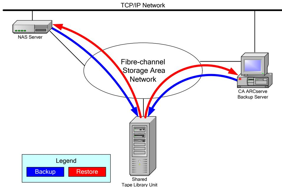
The following diagram shows an example of two or more NAS servers connected to the SAN that share a tape drive or TLU, and the CA ARCserve Backup server is not connected to the SAN.
