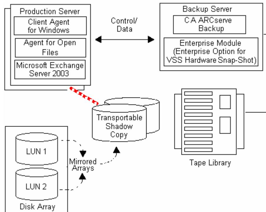
During backup operations, CA ARCserve Backup (the Requestor) contacts VSS on the production server and informs it to begin the transportable shadow copy process. VSS tells the Writer to prepare the data for the shadow copy.
