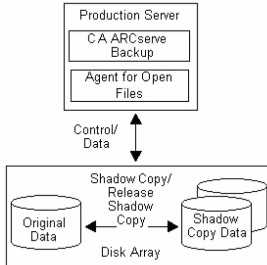
The following illustration displays remote configuration of the supported Client for VSS Software Snap-Shot:
