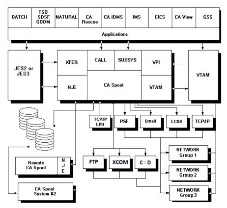
The following illustration shows how CA Spool is related to the other system components in an IBM z/OS environment.
