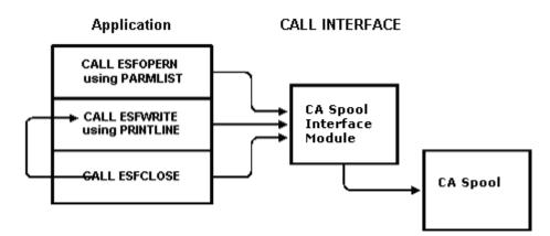
Application programs can interact with CA Spool by using the Call Interface; this interface uses all standard linkage conventions.
