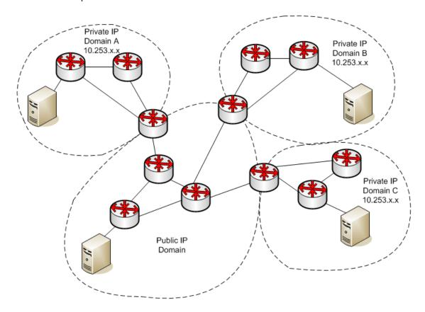
Domains can represent the managed network of a company, a newly acquired division of a large enterprise, or a managed wireless hot spot in an airport terminal.
