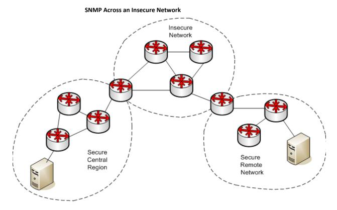
Secure Domain Manager lets network managers encrypt all management traffic that passes between the SpectroSERVER host and the host in the remote managed network. This solution securely passes insecure SNMP traffic across insecure networks. Data security is maintained when the traffic traverses the intermediate insecure networks.
