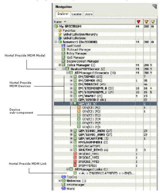
The following image displays an expanded view of Telco EMS Manager and its elements.
