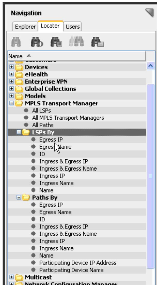
For example, if you know the IP address or name of a specific router, you can search for all LSP Paths that use it. Using the list of Paths affected by the router can be useful when performing scheduled maintenance. You can change your Paths to use a different router, or be sure that at least one secondary Path is provided for each LSP before the maintenance. Also, you can give prior notice to any customers affected by those Paths.
