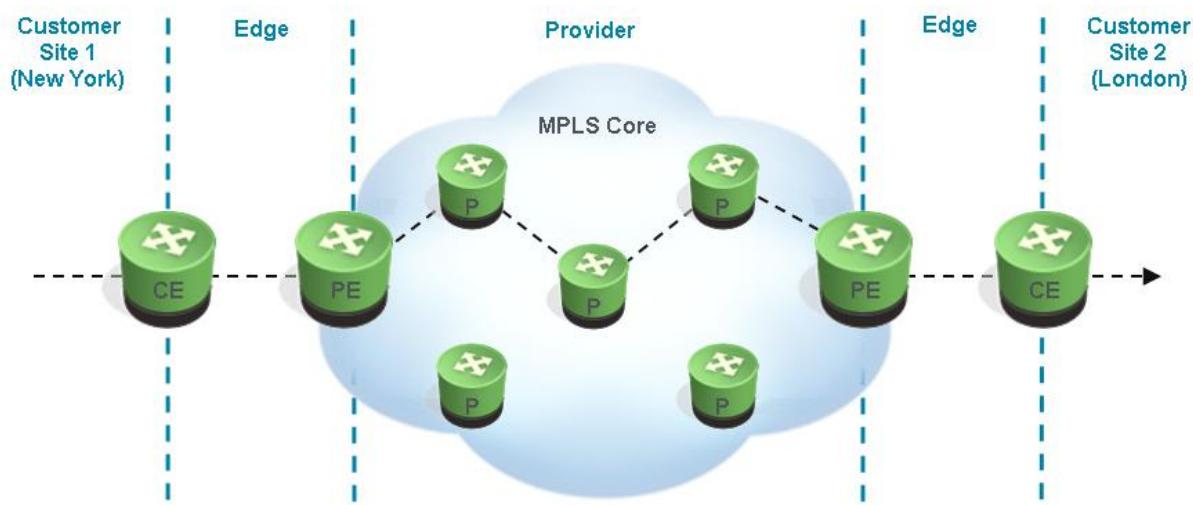
As shown in the diagram above, a customer communicates from one side of their network to the other using the Provider's MPLS network as follows:
