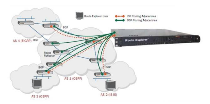
The routing analytics appliance is developed and marketed by CA's Technology Partner - Packet Design. This appliance operates by passively monitoring the routing protocols exchanges between routers. It 'announces' itself as if it was a router, but doesn't advertise any prefixes, so no traffic flows to/through it. Therefore, it's neither a bottleneck nor a failure point.
