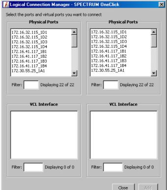
The dialog lists the physical ports on the ATM devices connected to the selected cloud, or connected to or contained within the selected network. Only the ports that currently have virtual link models are included in the lists.
