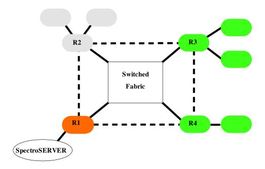
If, for example, R3 responds that it is available, but R1 does not respond, CA Spectrum creates a red alarm on R1 and changes R2 and the models that depend on its connectivity to gray to indicate a suppressed state.
