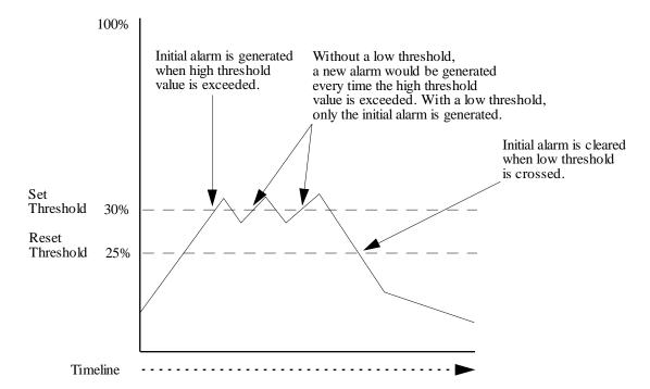
By default, the high thresholds are set to 90% and reset at 80%, and the low thresholds are set to 0 and reset at 0. In other words, the low thresholds are disabled. The threshold values are recalculated at every poll cycle and represent the average number per poll.
