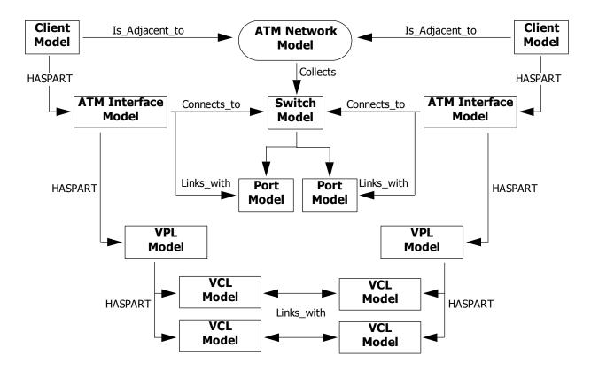
The following illustration shows the relationships between the modeled physical and virtual components in an ATM network.
