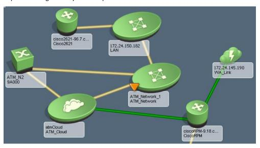
In a fully or partially meshed ATM network, each physical ATM interface may have logical connections with many other ATM devices. However, without ATM Circuit Manager, CA Spectrum's modeling functionality will only model physical ATM interfaces, leaving logical ATM interfaces unmanaged and limiting connectivity to physical links. Therefore, without ATM Circuit Manager, it is impossible to accurately represent the logical connectivity of the switches and routers in the ATM network.
