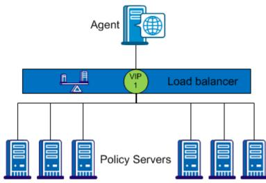
In the configuration shown in the previous diagram, the load balancer exposes multiple Policy Servers using a single VIP. This scenario presents a single point of failure if the load balancer handling the VIP fails.
