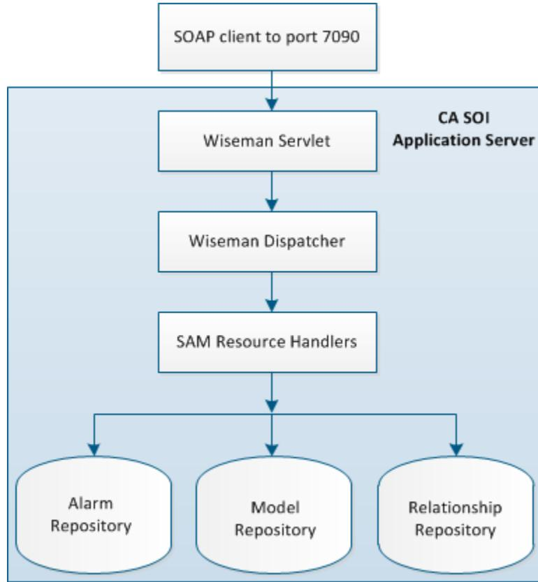
The WSManservlet intercepts client SOAP requests directed at the endpoint URL and dispatches them to the appropriate Resource Handler instance identified by the ResourceURI contained in the EPR element of the SOAP message. Wiseman automatically identifies the appropriate Resource Handler class in the following format: *Resource\_Handler.java*.
