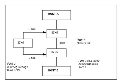
Rotate and backup links are not suitable for environments where the active sessions traverse different routes with widely differing transmission speeds. Take this into consideration when planning the COS definitions to be associated with the various sessions that form the INMC link.
