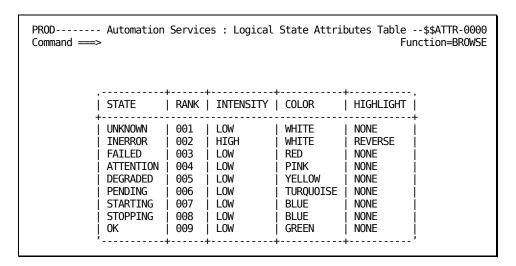
To display resources with a logical state of INERROR in red and reverse video at high intensity, you assign the following values:
