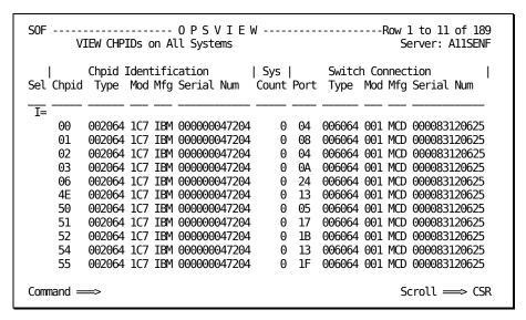
2. Enter line commands to display complete switch hardware ID, change the SOF switch name, display the ports for switch, display switch devices on connected systems, display CHPIDs connected to a switch.
