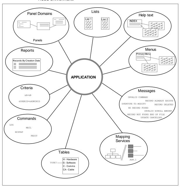
The following figure illustrates the components of an NCL application in the MODS environment.
