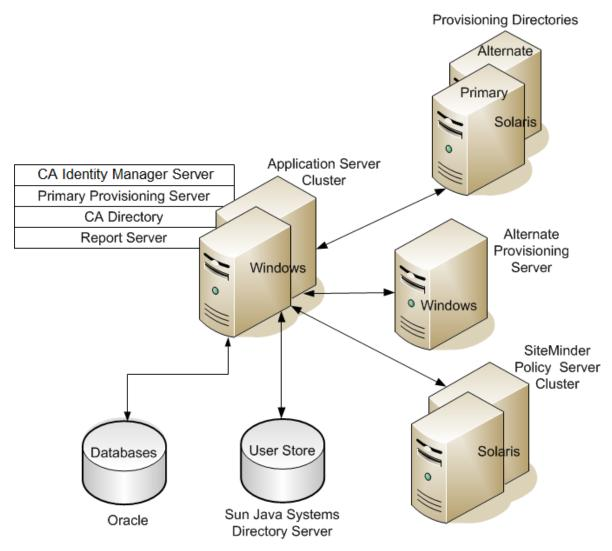
In addition to illustrating high availability, this figure shows the different platforms that are used for the components comparing to the SiteMinder illustration. For example, the database uses Oracle instead of Microsoft SQL Server, which appeared in the previous illustration.
