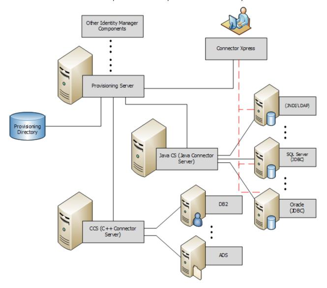
**Note:** The dashed red lines indicate that the direct communications between Connector Xpress and endpoints are read-only. These direct communications occur when setting up data sources.
