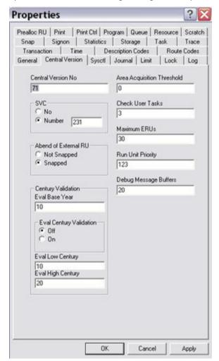
The Central Version tab in the following illustration on the system object has been updated to include the Debug Message Buffers parameter and Century Validation ones.
