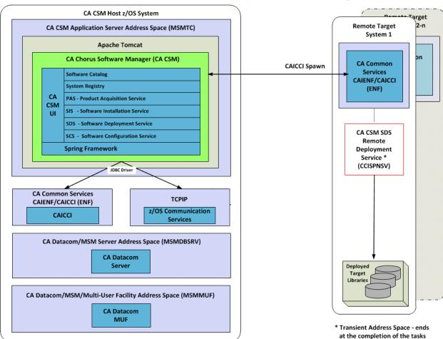
CA CSM on z/OS Host System with SDS Remote Deployment Service on Remote Target System
