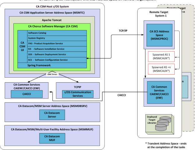
CA CSM on z/OS Host System with SCS Address Space on Remote Target System
