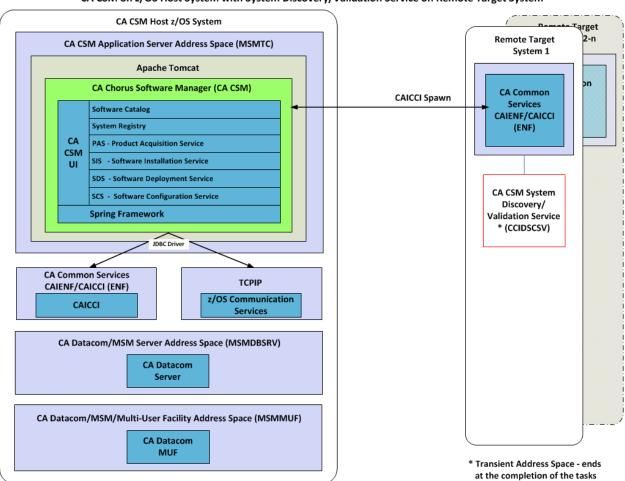
CA CSM on z/OS Host System with System Discovery/Validation Service on Remote Target System
