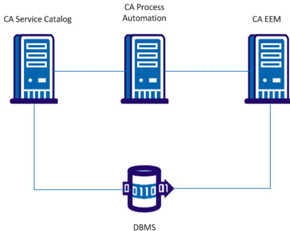
This model applies to systems with an expected average load of 1 to 10 catalog requests per minute. Clustering does *not* apply.
