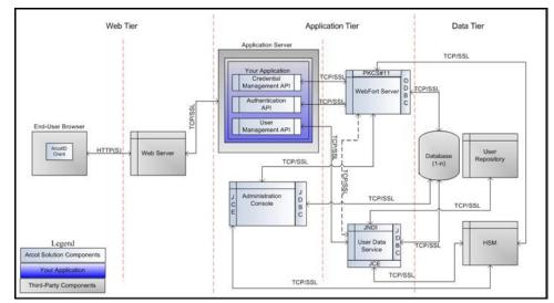
The following figure illustrates the possible communication modes that are supported between AuthMinder and its components.
