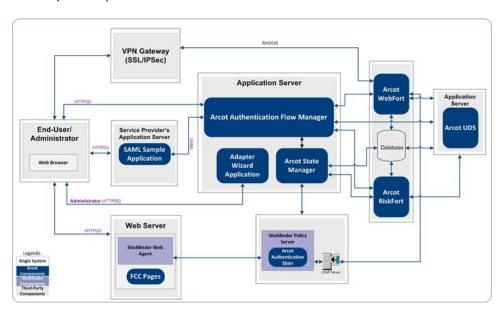
Install and deploy Adapter components as depicted in the preceding diagram. Also, CA recommends using a secured communication channel between all Adapter components. For more information about configuring SSL communication, see appendix, "Configuring SSL and Redirection in Apache Tomcat" (see page 163).
