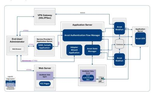
Install and deploy Adapter components as depicted in this figure. Also, it is recommended that you use a secured communication channel between all Adapter components. For more information about configuring SSL communication, see "Configuring SSL in Apache Tomcat" (see page 173).
