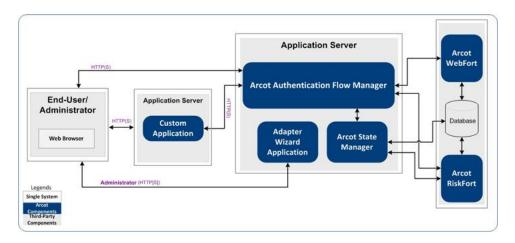
Install and deploy Custom Application and Adapter components as depicted in this figure.
