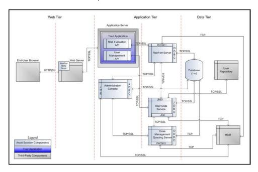
As shown in the figure, the default mode of communication between components is TCP, RiskMinder Server supports SSL communication (two-way and one-way) with the following components to ensure integrity and confidentiality of the data being exchanged during a transaction:
