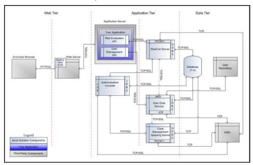
As shown in this figure, the default mode of communication between components is TCP, RiskMinder Server supports SSL communication (two-way as well as one-way) with the following components to ensure integrity and confidentiality of the data being exchanged during a transaction:
