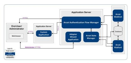
Install and deploy Custom Application and Adapter components as depicted in this figure.
