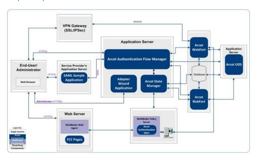
Install and deploy Adapter components as depicted in this figure. Also, it is recommended that you use a secured communication channel between all Adapter components. For more information about configuring SSL communication, see "Configuring SSL in Apache Tomcat" (see page 173).
