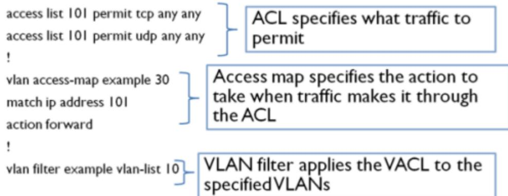
The VACL in the example is configured to deny ICMP traffic on VLAN 10. The ACL permits TCP and UDP traffic only, which implicitly denies all other Layer 3 traffic. The access map applies the ACL with a priority of 30 and specifies that traffic meeting the ACL is forwarded to its destination. The **vlan filter** command applies the access map to VLAN 10.
