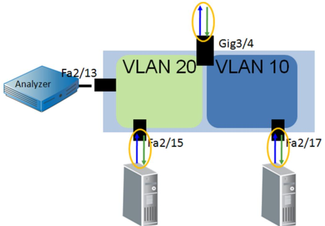
The preceding illustration shows a Layer 2 device that uses a trunk port to send traffic to a Layer 3 device. This configuration leads to duplication of all traffic between client and server and intra-VLAN. Also, traffic is quadruplicated when hosts in VLAN 10 and VLAN 20 communicate with each other.
