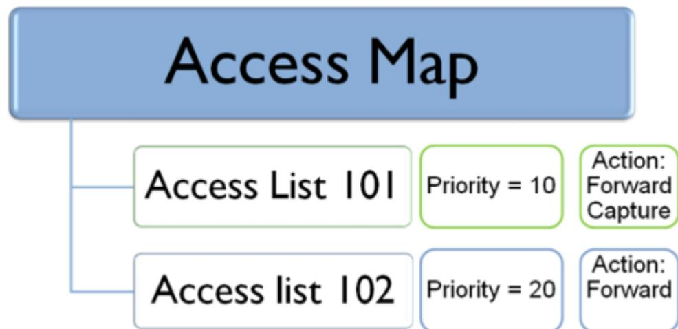
The preceding illustration depicts an access map that contains two ACLs. Each ACL is associated with a separate set of actions. The priority number determines which ACL is processed first (the lowest).
