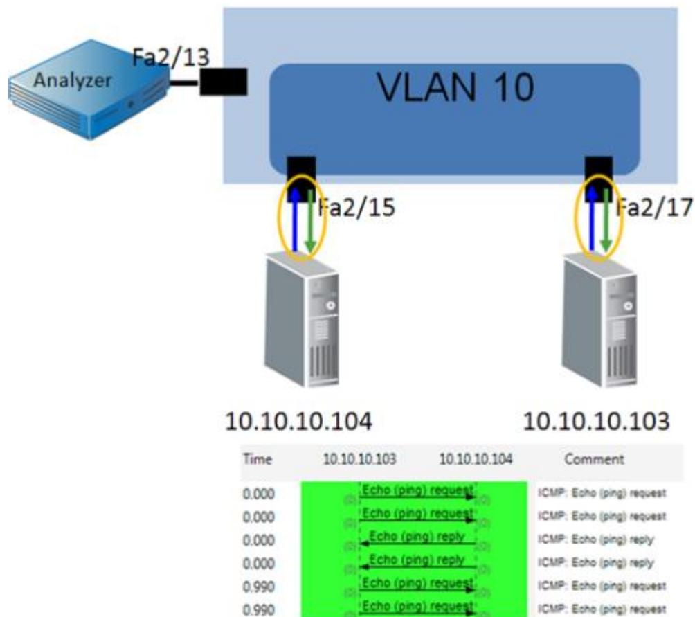
Duplication also occurs when more than one VLAN is sourced and servers in both VLANs communicate with each other. The following commands represent the configuration in the illustration:
