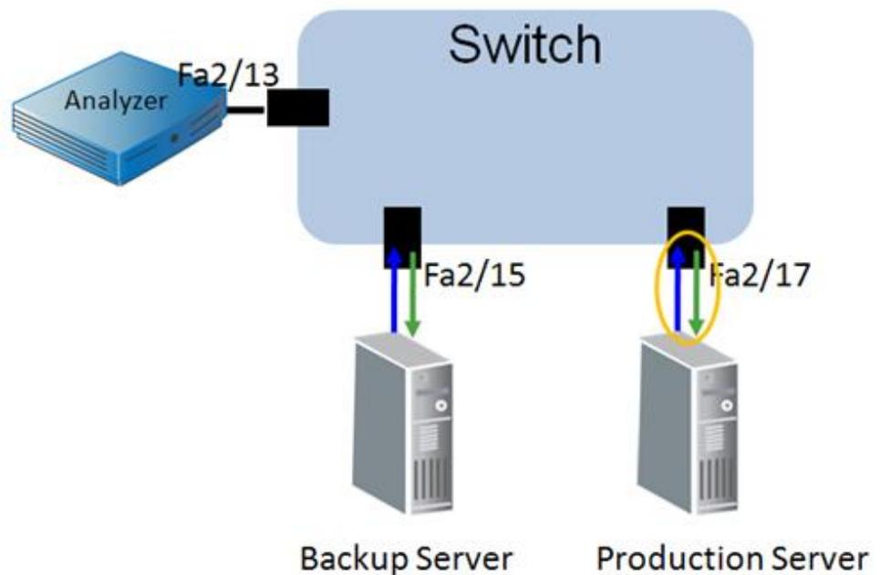
The configuration in the illustration captures all traffic to and from the production server, while ignoring traffic to and from the backup server. The following commands represent the configuration in the illustration:
