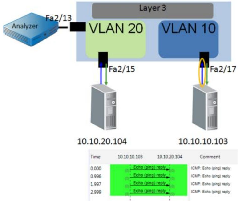
The preceding illustration shows that the SPAN configuration does not see traffic that enters VLAN 10 from Layer 3, because no physical interface is involved. Packets are seen only as they are received by an interface in VLAN 10. Packets destined for hosts in VLAN 10 (TX) are missed. Traffic coming from VLAN 20 or from end users is missed.
