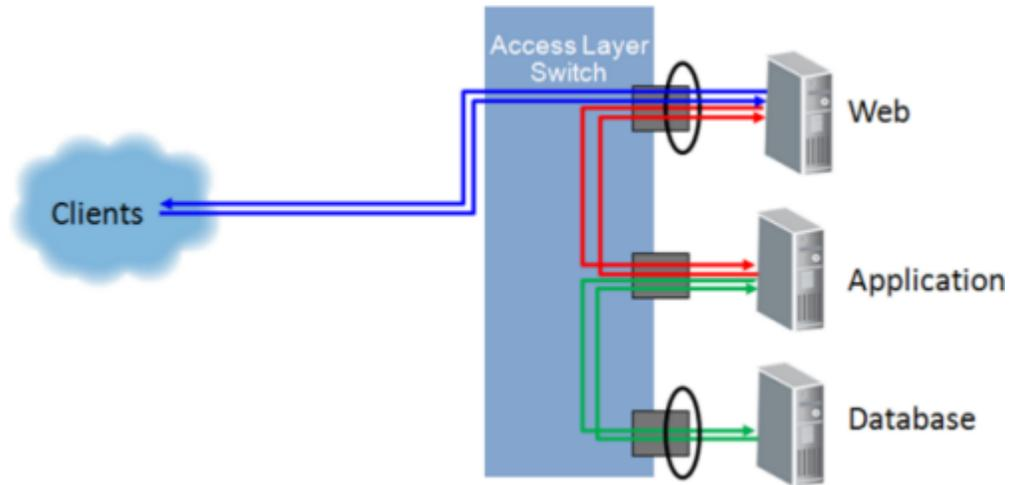
The preceding figure shows how to avoid packet duplication by sourcing the port mirror from every other tier of a multi-tiered application. Notice that each flow of data is only circled (sourced) once, and each flow crosses only one source port.
