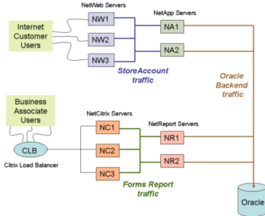
Because the mirroring configuration includes both transmitted and received packets, the number of ports required to be mirrored is reduced. When you mirror a tier, you see the traffic to that tier and to the next tier after it.
