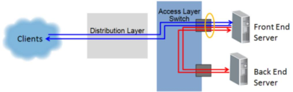
The preceding figure identifies the port to use as the source when a monitoring application talks between two servers. When the front-end server is the source, the monitoring application sees transmitted and received data at the client and at the back-end server. When more than two tiers are talking, use the interface of every alternate tier as a source.
