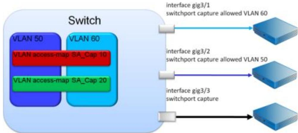
The preceding diagram shows how traffic is captured and filtered from VLANs 50 and 60. Three capture ports are configured, one to accept only VLAN 50, one to accept only VLAN 60, and a third to accept both VLANs.
