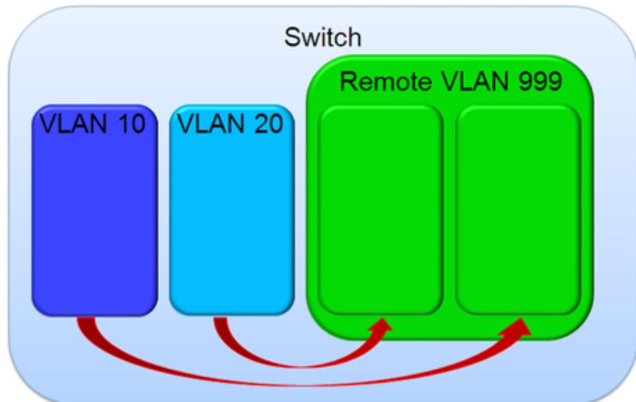
The preceding illustration shows how data from the source VLANs is copied to a new RSPAN VLAN. The following commands represent the configuration in the illustration:
