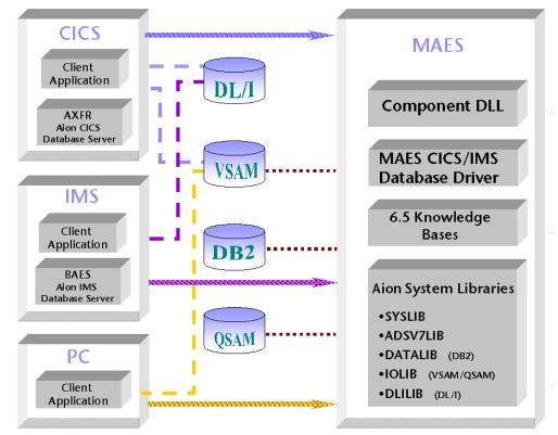
MAES provides the environment for running components on a mainframe server. When a client establishes an APPC/VTAM session to MAES, the following events occur:
