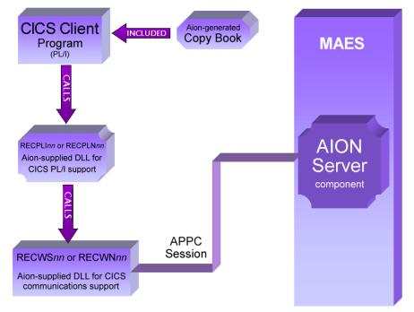
In the illustration, RECPLI*nn* is the Suspend version. The Non-Suspend version is named RECPLN*nn*. The Aion calls in the PL/I client program always specify RECPLI*nn*. The SDS file linked with the PL/I client determines whether RECPLI*nn* or RECPLN*nn* actually is invoked.
