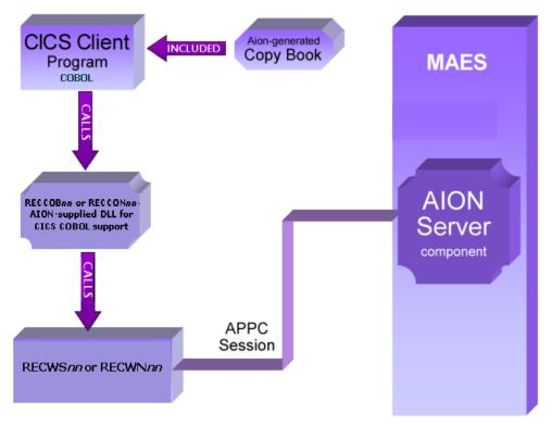
In the illustration, RECCOB*nn* is the Suspend version. The Non-Suspend version is named RECCON*nn*. The Aion calls in the COBOL client program always specify RECCOB*nn*. The SDS file linked with the COBOL client determines whether RECCOB*nn* or RECCON*nn* actually is invoked.
