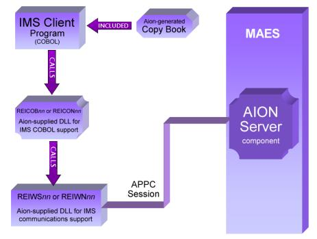
In the illustration, REICOB*nn* is the Suspend version. (The Non-Suspend version is named REICON*nn*. The Aion calls in the COBOL client program always specify REICOB*nn*. The SDS file linked with the COBOL client determines whether REICOB*nn* or REICON*nn* actually is invoked.
