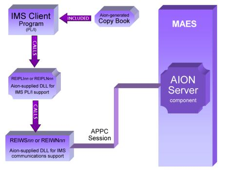
In the illustration, REIPLI*nn* is the Suspend version. (The Non-Suspend version is named REIPLN*nn*. The Aion calls in the PL/I client program always specify REIPLI*nn*. The SDS file linked with the PL/I client determines whether REIPLI*nn* or REIPLN*nn* actually is invoked.
