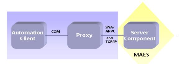
The Windows-based client uses the Microsoft COM interface. For each Aion mainframe application, an z/OS COM component (proxy) is generated which acts as a COM object. This COM object exports all classes and methods contained in the server component.
