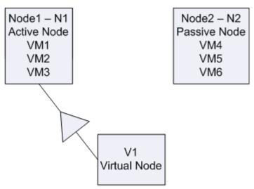
In an ideal scenario, virtual cluster node V1 directs network traffic to the active node (N1). When failover occurs, virtual cluster node V1 directs the network traffic to the passive node (N2), and all of the VMs in the active node (N1) move to the passive node (N2).
