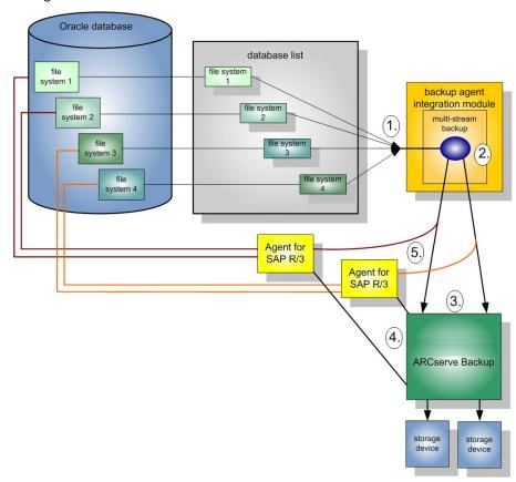
The following diagram illustrates data on four file systems being backed up to two storage devices:
