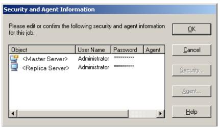
Each Arcserve Replication scenario displays two sets of credentials; one for the Master server and one for the associated Replica server. A graphic symbol next to the server name indicates if the server is a Master (active) server or a Replica (standby) server.
