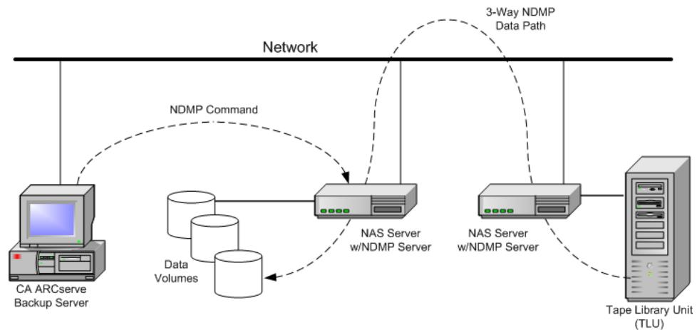
The following diagram shows an example of a NAS Filer to Server restore:
