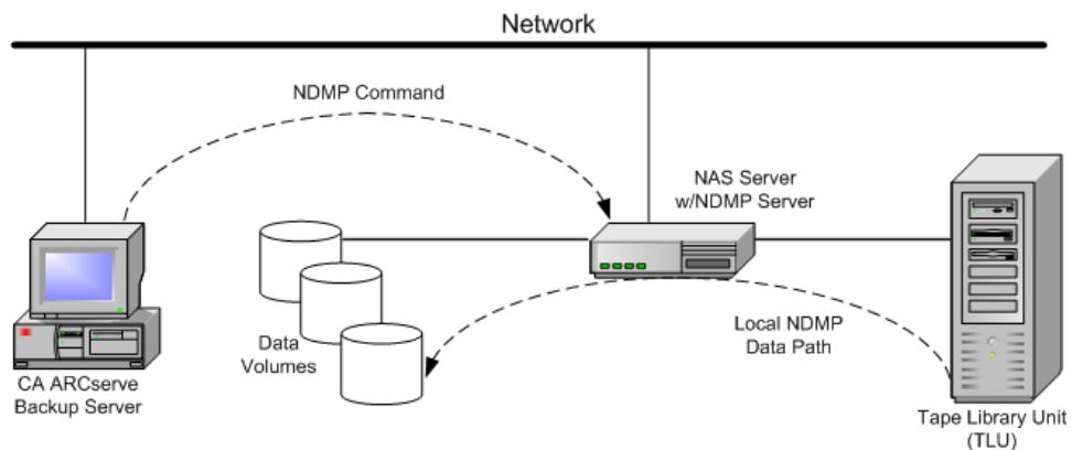
The following diagram shows an example of a three-way restore:
