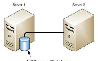
ARCserve Database (Local copy not retained on Server 2) In the following diagram, multiple Arcserve Backup servers are sharing a centralized database. A copy of the Arcserve Backup database is retained on one of the servers sharing the database.
